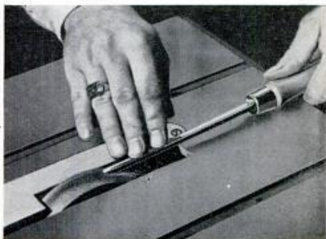
Above, same setup on the circular-saw table. Wheel is adjusted for height by raising saw arbor. Below, gouge is supported on table and rolled freehand
